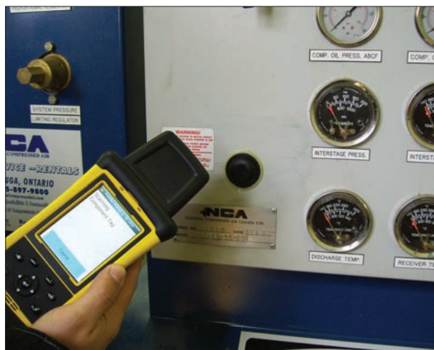
At the drilling sites, Nabors' field workers use handheld interrogators that connect to a back-end server via satellite communications.
